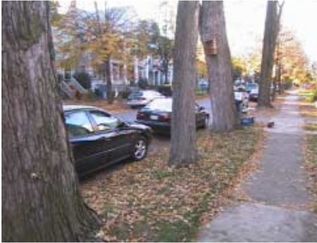
A five foot wide sidewalk offset from the curb line by six feet provides a functional and comfortable walking environment.
